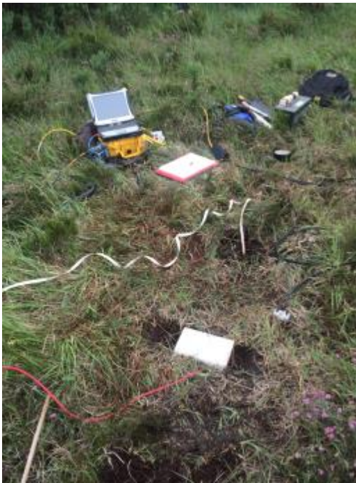
Figure 9. Downhole sonde and shear wave source
