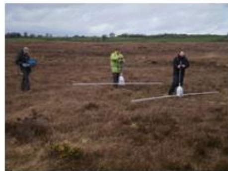
Figure 1. Investigation of peat with GPR (top) man-hauling 250 MHz equipment (middle) all-terrain vehicle with 100 MHz unit (bottom) variable frequency antennae.
