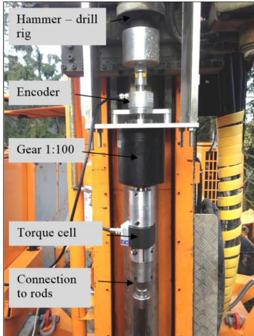
Figure 2 NTNU vane shear device
