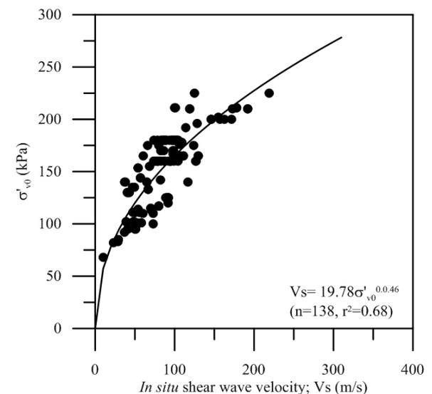
Figure 7 In situ  $V_s$  against vertical effective stress for all sites in the database.
