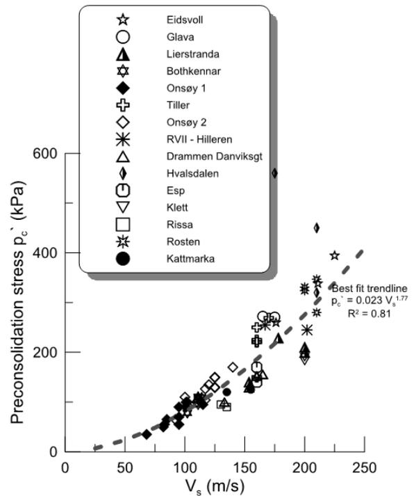
Figure 15 Results of  $p_c'$  versus in situ  $V_s$ .
