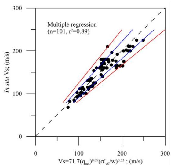
Figure 10 Comparison of measured and predicted  $V_s$  as a function of  $q_{net}$ ,  $\sigma'_{v0}$  and  $w$ . Blue lines show +/-10% envelope while red lines show +/- 20%.
