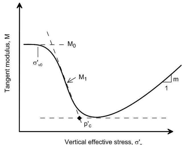
Figure 12 NGI's interpretation of the classical Janbu tangent modulus versus stress model.
