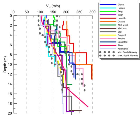
Figure 6 In situ shear wave velocity profile for sites in the Trondheim region.
