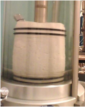
Figure 8 Specimen shape at failure ( \varepsilon_l = 10\% ) for B34 (B), Type 3, H/D=1 , D = 70\text{mm} .
