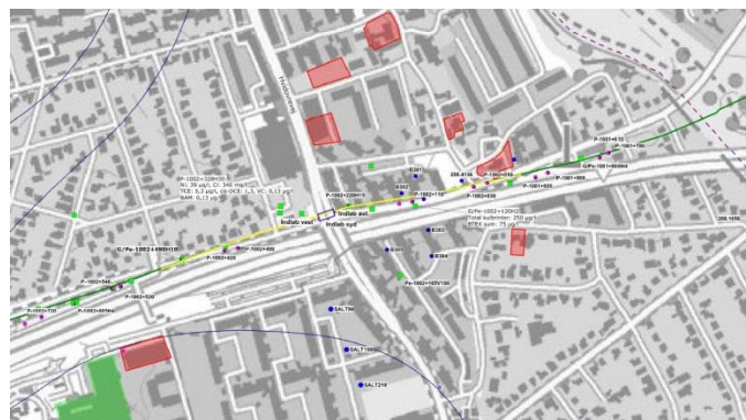
Figure 2 Location plan showing Hvidovre Tunnel and troughs, investigation boreholes and contaminated sites in Hvidovre Municipality.
