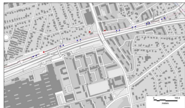
Figure 5 Map showing location of wells used for pumping tests and flow logs around the centre of the Hvidovre Tunnel. Blue dots denote wells used for pumping tests and red dots denote wells used for flow logging.
