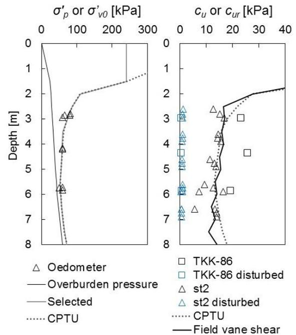
Figure 2 Left: Preconsolidation pressure ( $\sigma'_p$ ) and effective overburden pressure ( $\sigma'_{vo}$ ) versus depth. Right: Undrained shear strength ( $c_u$ ) and remoulded undrained shear strength ( $c_{ur}$ ) versus depth.
