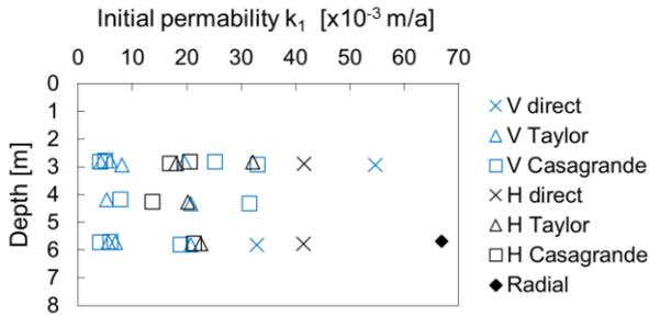
Figure 4 Initial vertical (V), horizontal (H) and radial permeability versus depth.
