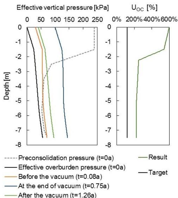
Figure 6 Left: Preconsolidation pressure, effective overburden pressure and; effective vertical pressure before, at the end and after the vacuum. Right: Degree of overconsolidation; target and the result.
