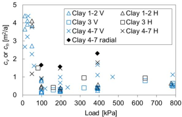
Figure 3 Vertical and horizontal coefficients of consolidation ( $c_v$  and  $c_h$ ) at different load increments and layers.
