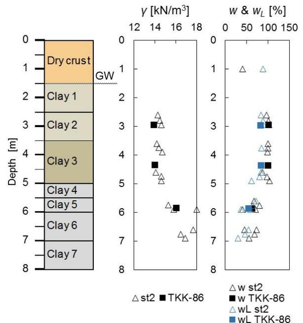
Figure 1 Soil layers, unit weight ( $\gamma$ ), water content ( $w$ ) and liquid limit ( $w_L$ ) from different samplers.
