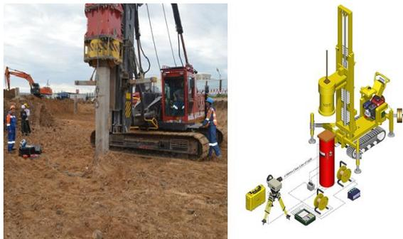
Figure 4 Photo and schema of dynamic load testing in Kazakhstan.
