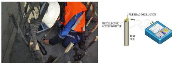
Figure 11 Photo and schema of pile integrity testing in Kazakhstan.
