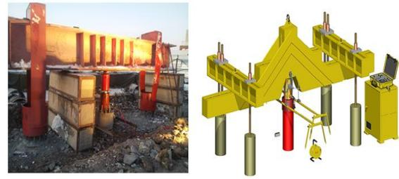
Figure 5 Photo and schema of static load testing in Kazakhstan.
