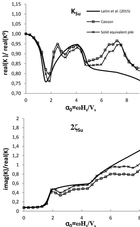
Figure 7 Variation of the translational stiffness and damping coefficients with respect to the dimensionless frequency for profile 2.
