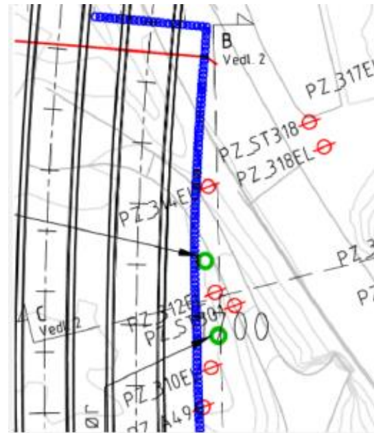
Figure 9 Location of the pump wells and piezometers in connection with the full scale pumping trials.
