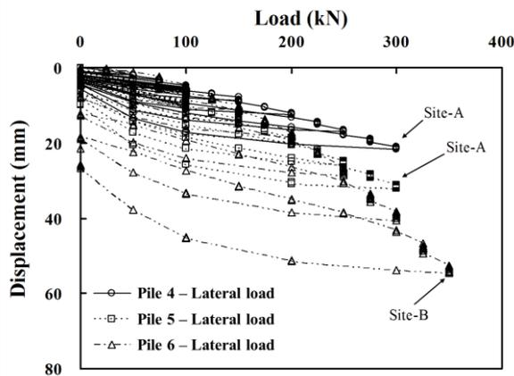
Figure 3 Load-settlement relation of lateral load tests.
