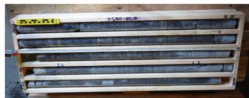
Figure 9 Actual core box. It is possible to see that the core stored in a 1m run is not always the full length, as it is clear in the lower three runs
