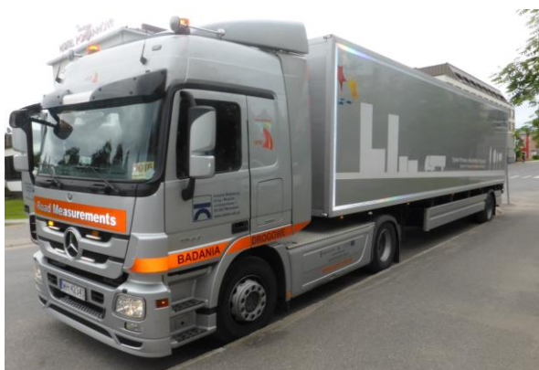
Figure 2. TSD truck used deflection surveys in Finland.
