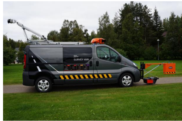
Figure 1. Road survey system equipped with ground penetrating radar system (in front) and a 2D laser scanner (at the back).
