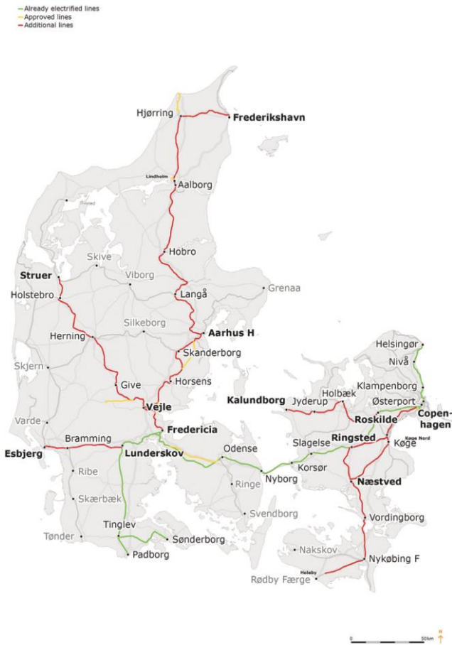
Figure 1, A map of Denmark showing the extent of the planned works with red and yellow lines. Green lines represent already electrified railway sections.
