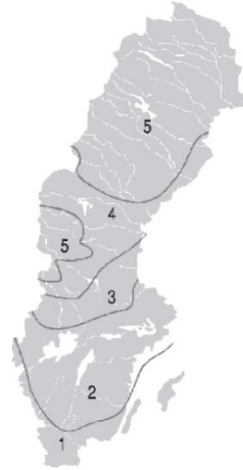
Figure 4 The five climate zones in Sweden used for frost design of pavements. Trafikverket, (2011).
