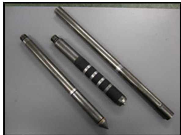
Figure 2 Example of R-CPTU probe (NIFS-report 2015-126).
