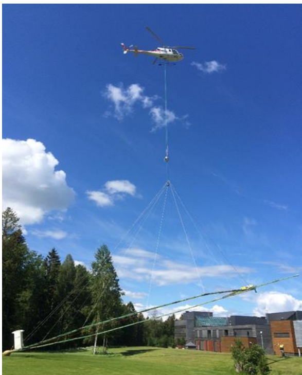
Figure 5 Equipment for AEM measurements (NIFS report 2015-126).
