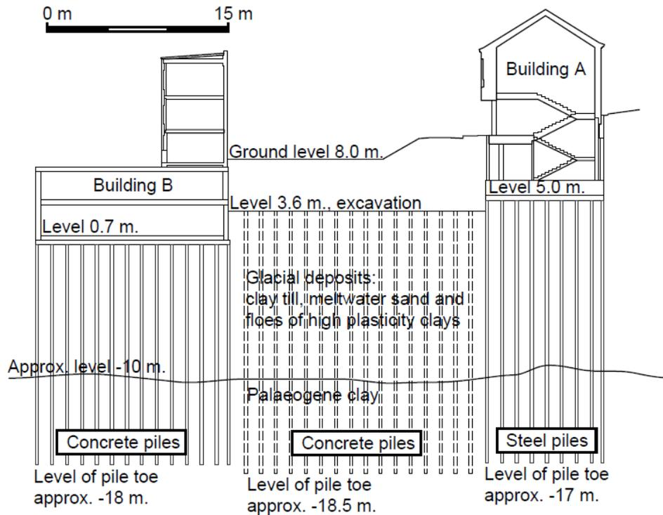
Figure 3 Cross section of the basement excavation for Aarhus Story and the adjacent buildings (Southeast to North-western direction).
