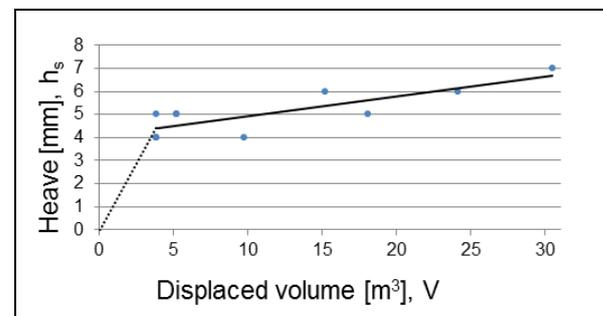
Figure 7 A linear correlation between heave and displaced volume for distances up to 11 m, with a relative distance  $s/L=0.05-0.5$ . The trend line is given by  $h_s=0.085 \cdot V+4$  for  $V=4m^3-30m^3$ .
