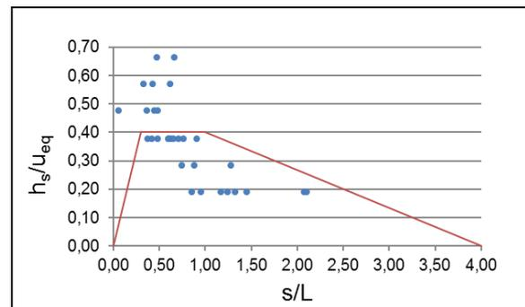
Figure 8 The data from this case study (blue) compared with the model suggested by Wersäll and Massarsch (2013) (red). The data is for displaced volume  $V=4\text{ m}^3-30\text{ m}^3$ .
