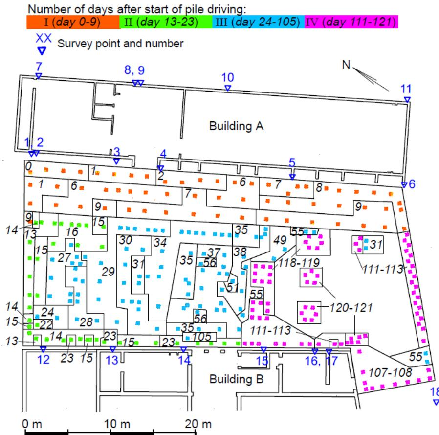
Figure 4 The progress of pile driving at Aarhus Story.
