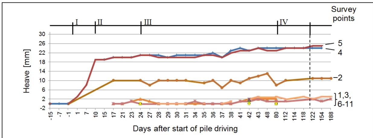
Figure 5 Accumulated relative heave of Building A with an indication of the pile driving periods. The timeline indicates all days on which measurements are made, represented by days after start of pile driving. End of pile driving is on day 121.
