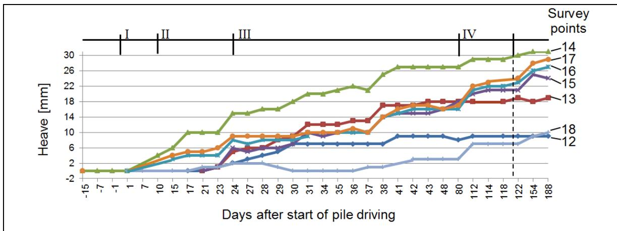
Figure 6 Accumulated relative heave of Building B with an indication of the pile driving periods. The timeline indicates all days on which measurements are made, represented by days after start of pile driving. End of pile driving is on day 121.
