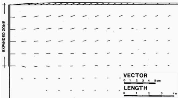
Figure 1 Soil displacement pattern around a driven pile, showing displacement vectors (Wersäll and Massarsch (2013)).
