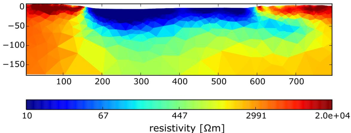
Figure 4: Inversion result of the ERT data set at Äspö HRL.
