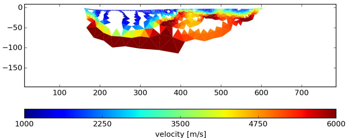
Figure 5: Inversion result of the seismic survey at Äspö HRL
